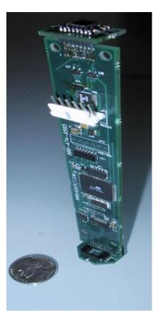
Low cost VERTICAL SOLID STATE advanced Pitch / Roll / Temperature compensated COMPASS / MAGNETOMETER system is built around a state of the art CMOS microcontroller utilizing AOSI's proprietary algorithm on a 0.9"DIAM x 6" assembled PCB is designed to fit sub 1" tubular probes.
